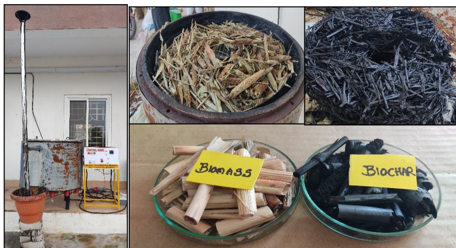
Fig 1: Electrical bin used for making biochar and biochar obtained from pearl millet straw
