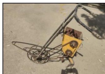
Fig 2: Manually operated garlic planter
