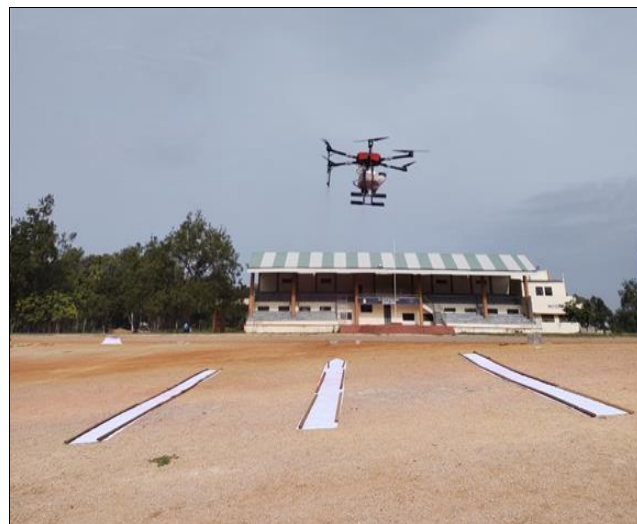
Fig 2: Operating drone mounted sprayer on white kraft paper roll to measure swath width
