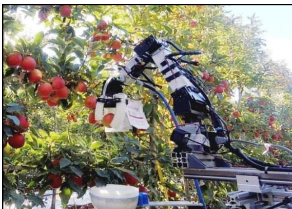
Fig 3: Robotic apple harvesting system with a 3D-printed soft robotic end effector (Hohimer et al. , 2019) [14]
