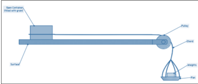
Fig 3: Experimental Setup for Coefficient of Friction
