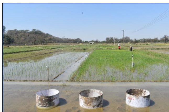
Fig 1: Drums arranged in experimental field to measure field water balance components
