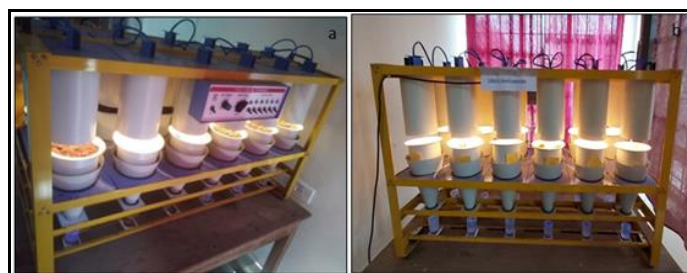
Plate 1: Tullgren funnels extractor (Soil Mesofauna Extractor)
