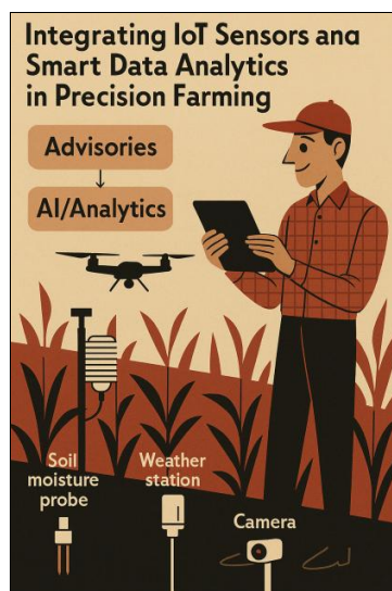
Fig 1: Integrating IoT sensors and smart data analytics in precision farming. IoT devices (bottom) measure environmental variables and crop status, while AI/analytics (center) generate advisories (top). Sensors depicted include soil moisture probes, weather station, drones, cameras.
