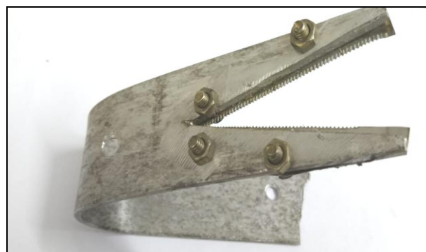
Fig 2: V-shape serrated cutter
