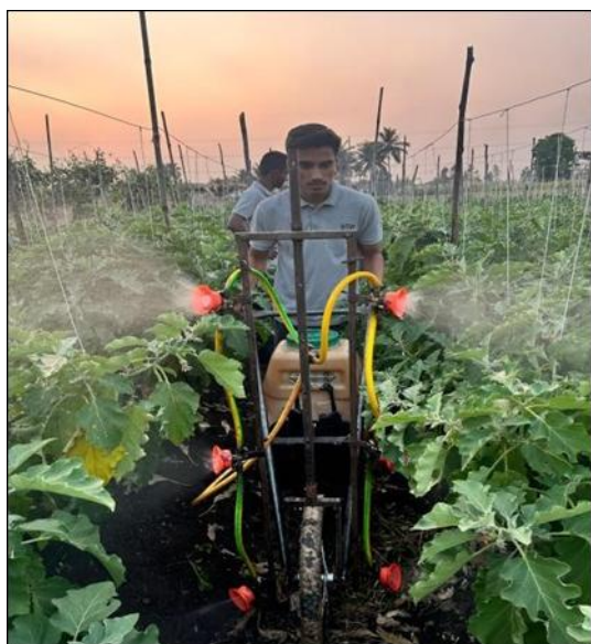
Plate 5: Spraying on brinjal crop using developed Engine operated walk type sprayer
