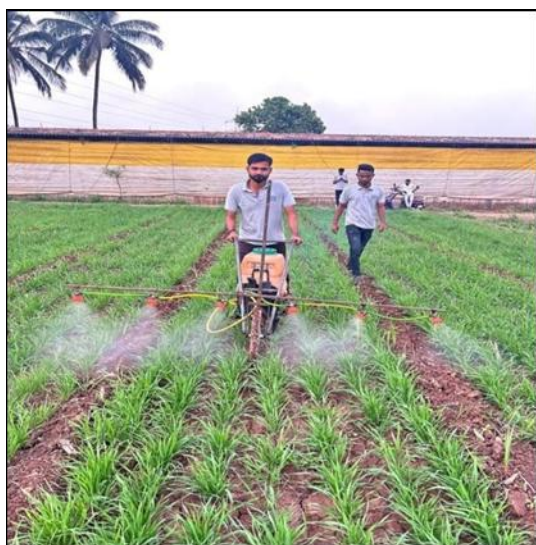
Plate 6: Spraying on wheat crop using developed Engine operated walk type sprayer
